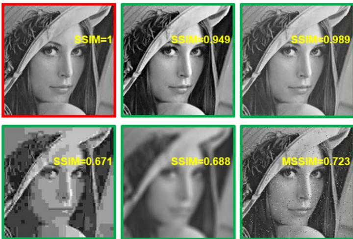
Figure 7.1-1. Relative to the standard image (in the red box), the five compromised images (in the green box) all have a MSE of 225 but look very differently. On the other hand, the SSIM measure (in yellow to be explained below) effectively reflects the visual quality.
